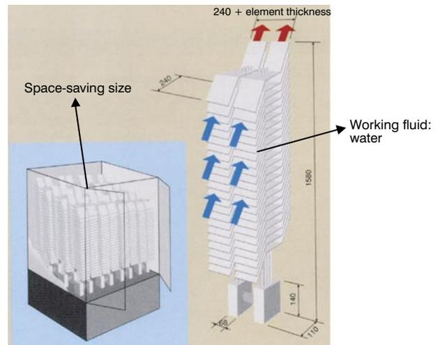
Figure 3 Cooling mechanism for HP-VAH.
