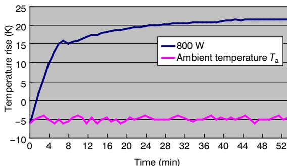
**Figure 6 Low-temperature start-up characteristics of HP-VAH.**
