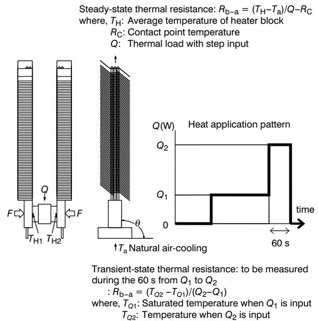
**Figure 4** Evaluation method of thermal characteristics of HP-VAH.
