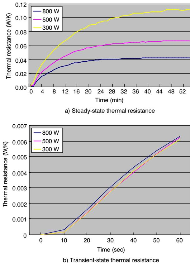
**Figure 5 Thermal resistance of HP-VAH.**
