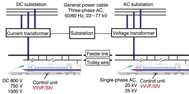
**Figure 1** Power control system at electric railway substations in Japan.
