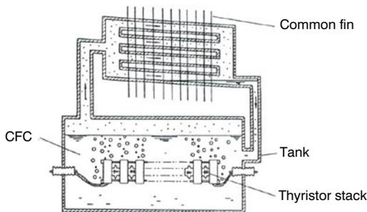
**Figure 2** Schematic of CFC boiling-tank cooling system conventionally used.
